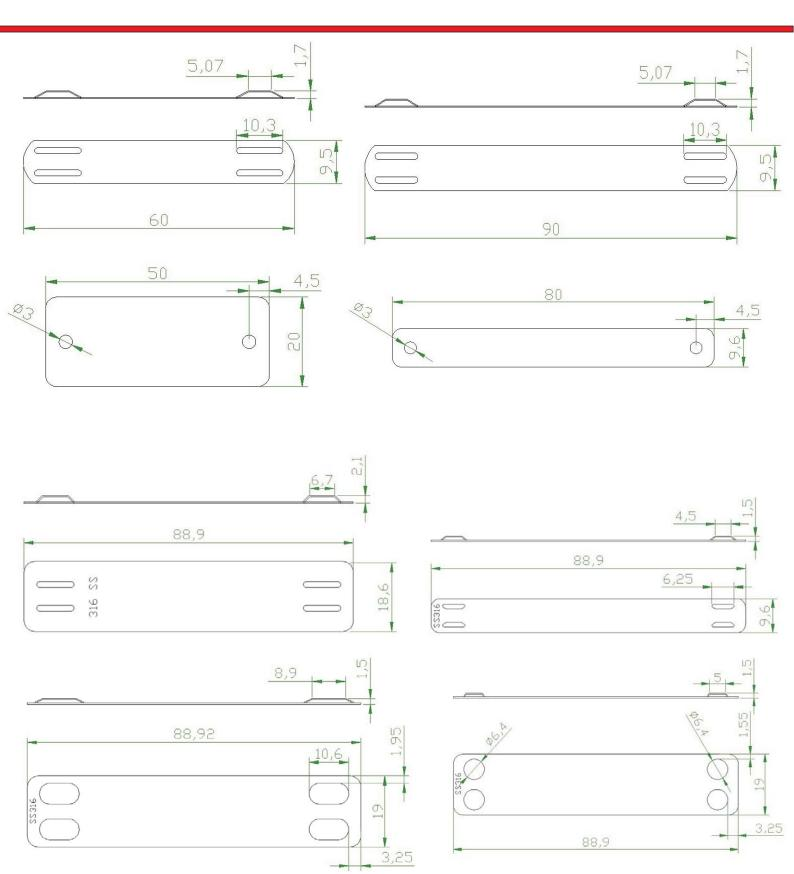
Material: 316# grade Stainless steel, 304 was optional for customer It could be embossed and its size could be designed as per request
